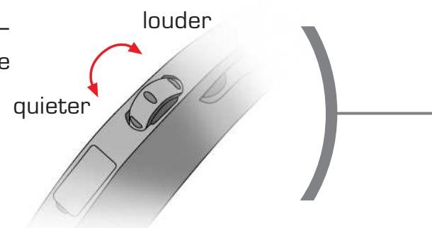
Systems with i-com technology automatically transfer volume change at one instrument to the second instrument.
